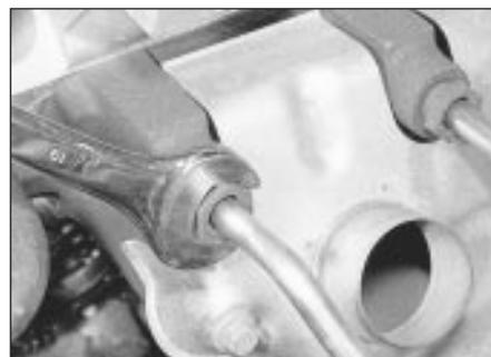
22.4 Unscrewing a pulse-air delivery tube union
