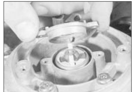
16.5b Removing the injector retaining collar
