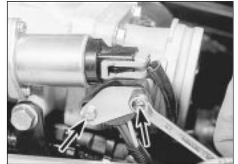
27.3 Unscrewing the throttle position sensor retaining bolts
