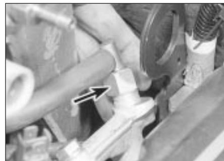
6.9 Fuel rail fuel feed union (arrowed)
