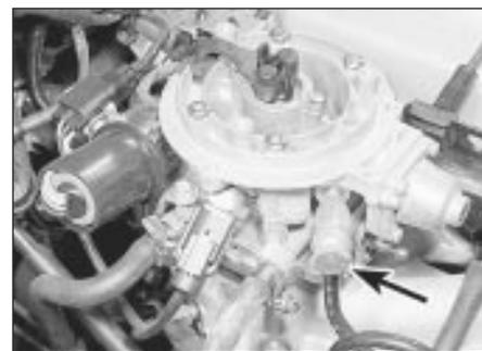
**4.4 CFI unit fuel inlet union (arrowed)**
