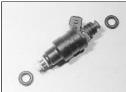
18.12 Fuel injector with seals removed
