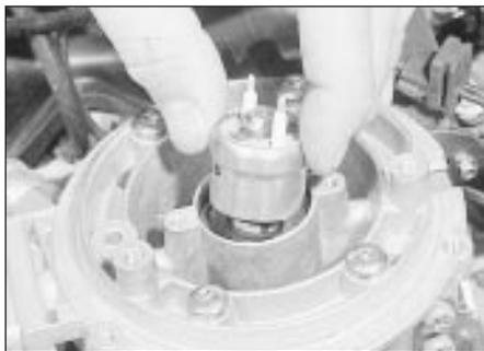
16.6 Withdrawing the fuel injector
