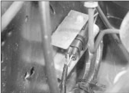
17.1 Fuel injector ballast resistor location (arrowed)
