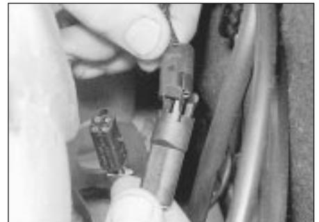
30.6 Disconnecting a fuel injection harness wiring plug
