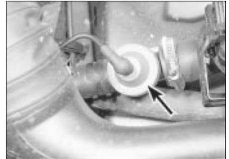
21.1 Pulse air system vacuum-operated air valve (arrowed)
