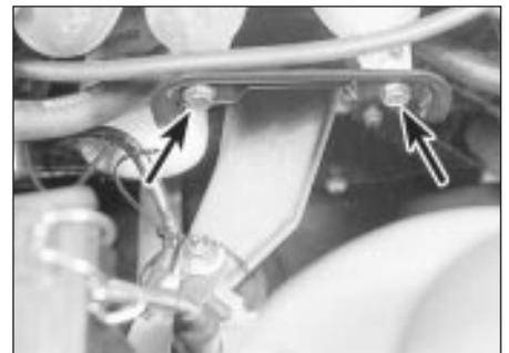
30.12 Lower inlet manifold bracket (arrowed)
