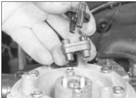
16.4 Disconnecting the fuel injector wiring plug
