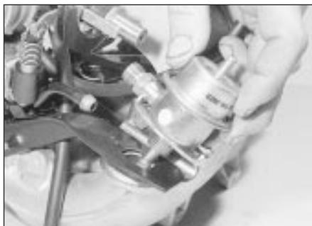
6.5 Withdrawing the fuel pressure regulator
